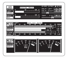
Not only can you specify time delay in feet or meters but simultaneously compensate for ambient temperature which affects sound speed!
